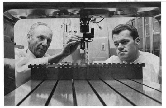
APPRENTICE ON THE JOB—Chuck Shinneman (8129), left, explains the operation of the two-coordinate measuring machine in Sandia/Livermore's Metrology Laboratory to apprentice Jim Nickerson. On-the-job training is part of a new mechanical measurment technician apprenticeship program, one of several technician apprenticeship programs established recently at Livermore.
